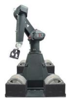
**Bolt**<sup>™</sup> **On Pedestal** has a stationary base which you either hold down with weights or, for more permanent installations, attach to the floor.
