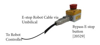
Bypassing the Universal E-stop System is for temporary use only. Robot will enable as soon as E-stop button is reset. This will also bypass the software E-stop and any other hardware E-stops and the robot will have no controlled E-stop action.
