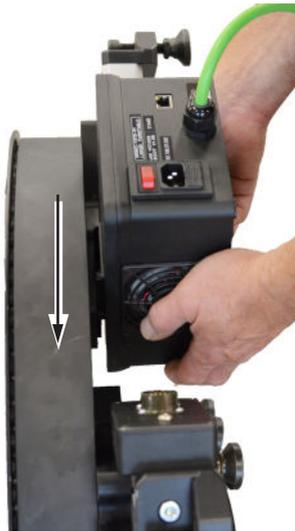
2. Use an hex key to tighten the grub screw to secure the control box to the Large Turntable.
