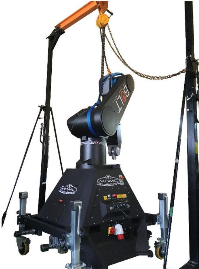
6. Wheel the Studiobot to the location and lower the 4 x feet to secure to the ground.
