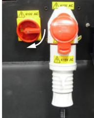
The Studiobot XL power-up sequence takes about three minutes. When it has completed, the Stäubli CS8 shows an “A” on its display.
