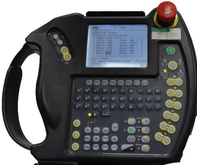
16. In the following example, the Roll limits have been modified to -720 to +720.
