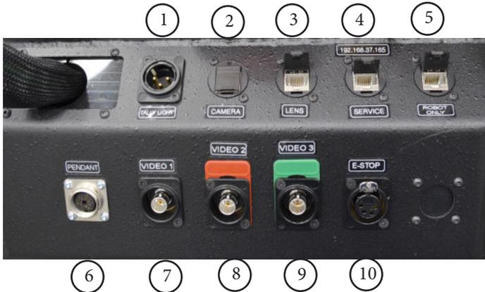
1. **TALLY LIGHT** connector is the power in connector for teleprompter.
