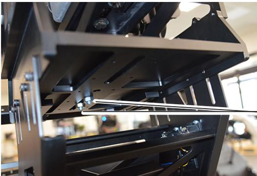
Screw the camera plate to the camera platform
