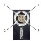
box which is set during manufacture. DSLR applications typically use two trigger outputs, on pins 2 and 3; one for shutter and one for auto-focus. Video applications typically use pin 2 for trigger output and pin 3 for trigger input.
