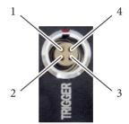
box which is set during manufacture. DSLR applications typically use two trigger outputs, on pins 2 and 3; one for shutter and one for auto-focus. Video applications typically use pin 2 for trigger output and pin 3 for trigger input.
