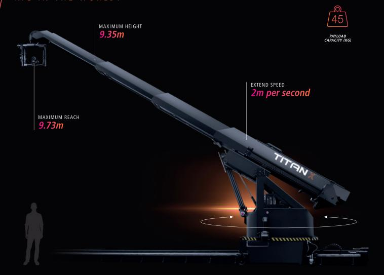
The Titan X has a huge 7m telescopic arm, capable of moving 2m per second – giving a 10m reach from the centre of the rig. The extremely fast base moves 3m per second on track; the two combined with rotate give you blistering camera speeds and creativity with maximum reach!
